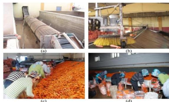
Fig. 1. Washing and conveyor belt (a), dispenser brush (b), sorting and packaging of carrots by workers (c, d)
