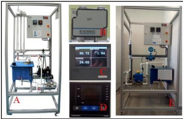
Fig. 1. a) LLCS, b) differential pressure sensor, c) recorder, d) process controller and e) FRCS
