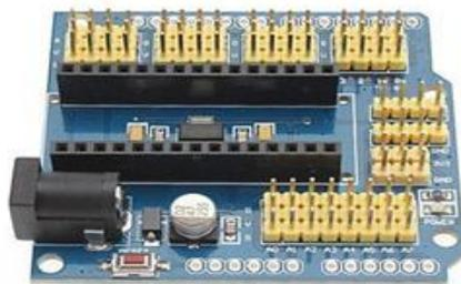
Fig. 8. Arduino Nano Sensor Shield
