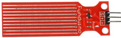
Fig. 5. Water Level Sensor
